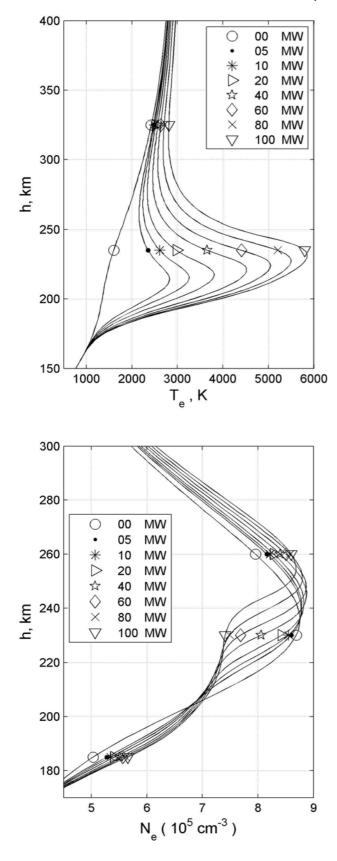
**Fig.1.** Profiles of the electron temperature versus distance from the Earth along the geomagnetic field line situated in the illuminated region at the moment of 300 sec after turn on. The results are given for different values of the EAP: 5, 10, 20, 40, 60, 80, and 100 MW, with symbol 0 MW indicating the results obtained under natural conditions without heating.
