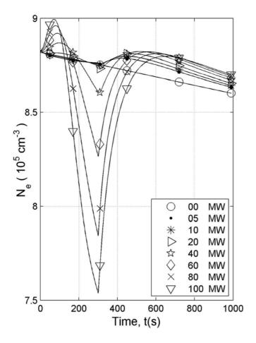
**Fig.3.** The time variations of the electron concentration (in units of  $10^5$  cm<sup>-3</sup>) at the level h=235 km. The results are given for different values of the EAP: 5, 10, 20, 40, 60, 80, and 100 MW, with symbol 0 MW indicating the results obtained under natural conditions without heating.
